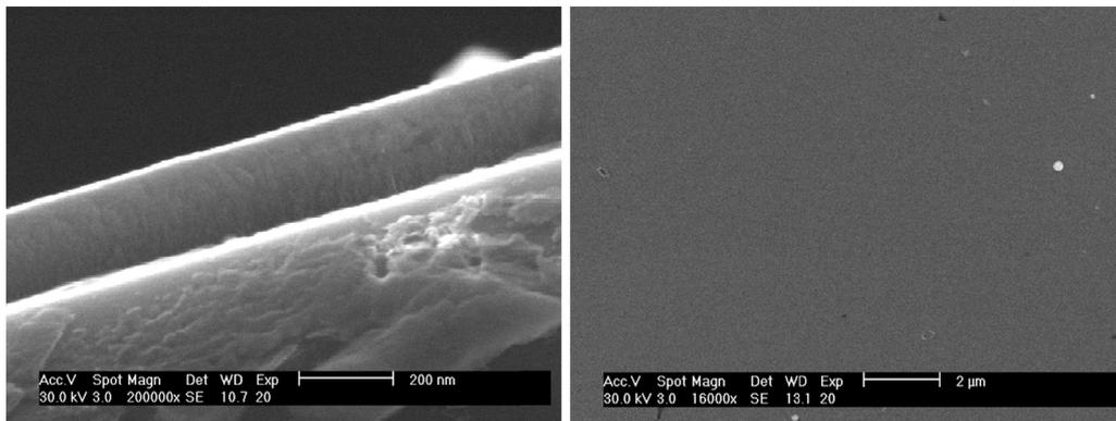
**Fig. 2.** SEM images of a fractured ZrN film and its surface.
