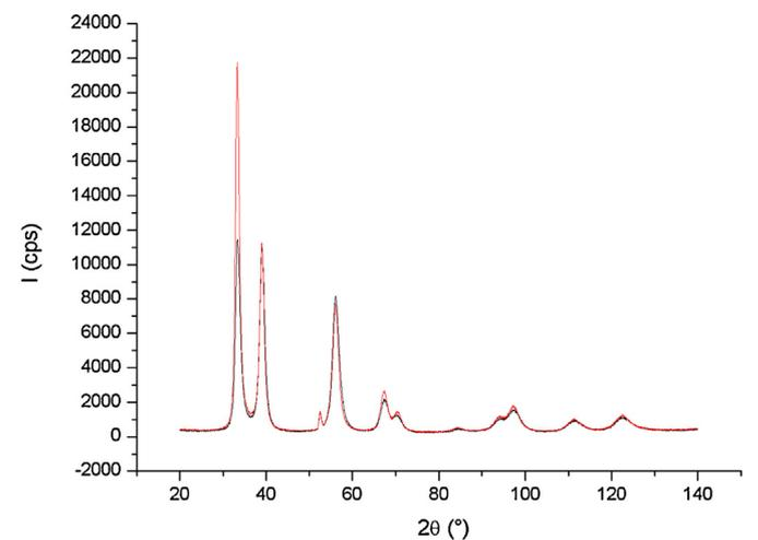
**Fig. 4.** Comparison between the diffraction patterns collected on ZrN samples irradiated at two distinct fluences (black  $10^{14} \text{ cm}^{-2}$ ; red:  $10^{15} \text{ cm}^{-2}$ ) under an incidence angle of  $1^\circ$ . (For interpretation of the references to color in this figure legend, the reader is referred to the web version of this article.)
