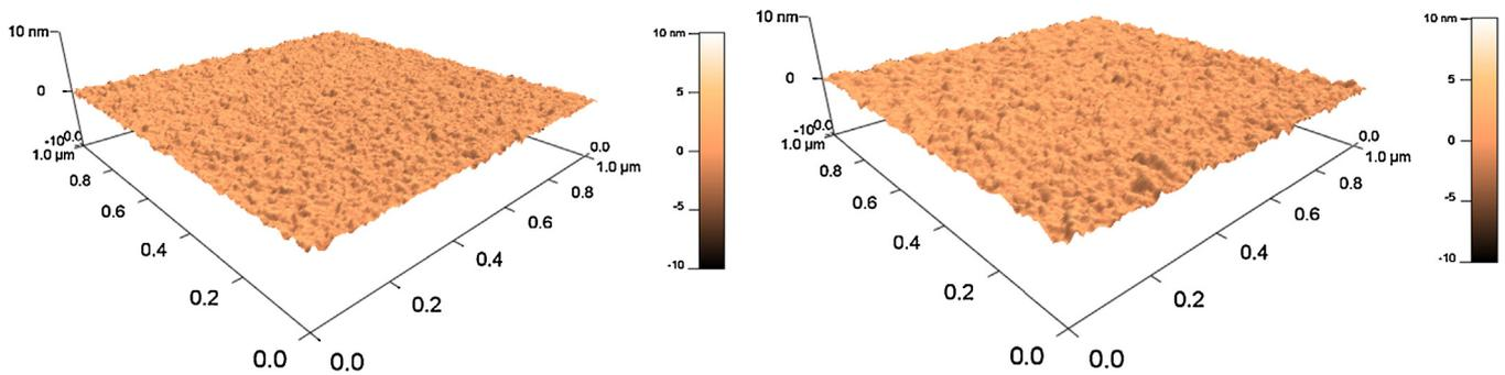
**Fig. 1.** AFM images of the surface morphology of ZrN1 (left) and ZrN3 (right) as-deposited films.
