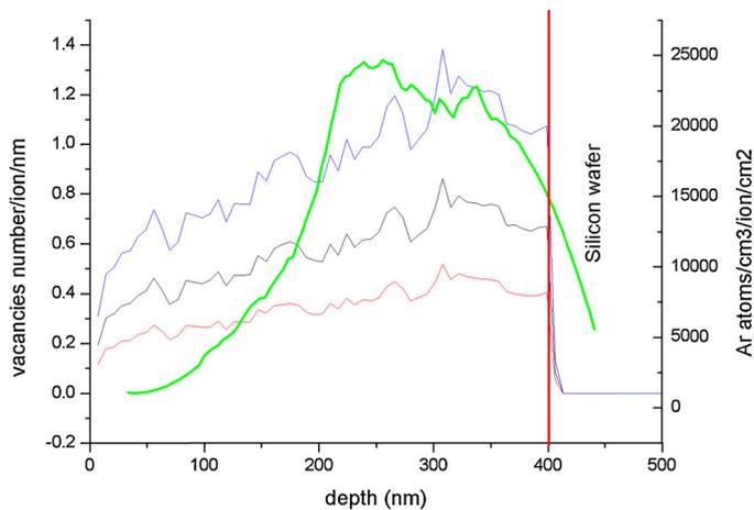
**Fig. 3.** SRIM calculations of the amount of Zr and N vacancies (red and black line, respectively; blue line indicates the total number of vacancies) created into Zr and N lattices as a function of the depth for 800 keV Ar ion irradiation. Atomic fraction of Ar ions implanted in the thin film is also plotted by the green curve. (For interpretation of the references to color in this figure legend, the reader is referred to the web version of this article.)
